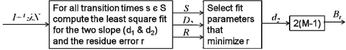
Figure 5: Block diagram of the nonlinear divergence estimator in the NLDE filter
