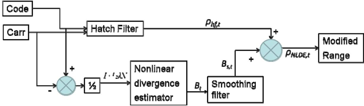
Figure 4: Block diagram of the NLDE filter
